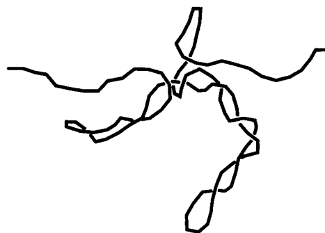
FIGURE 4 Simulated conformation of the DNA model for \sigma = 0.05 , f = 0.2 pN, and 200 mM concentration of monovalent salt. The molecule is nearly entirely plectonemically interwound: the applied force is insufficient to convert the supercoil into extended DNA.
